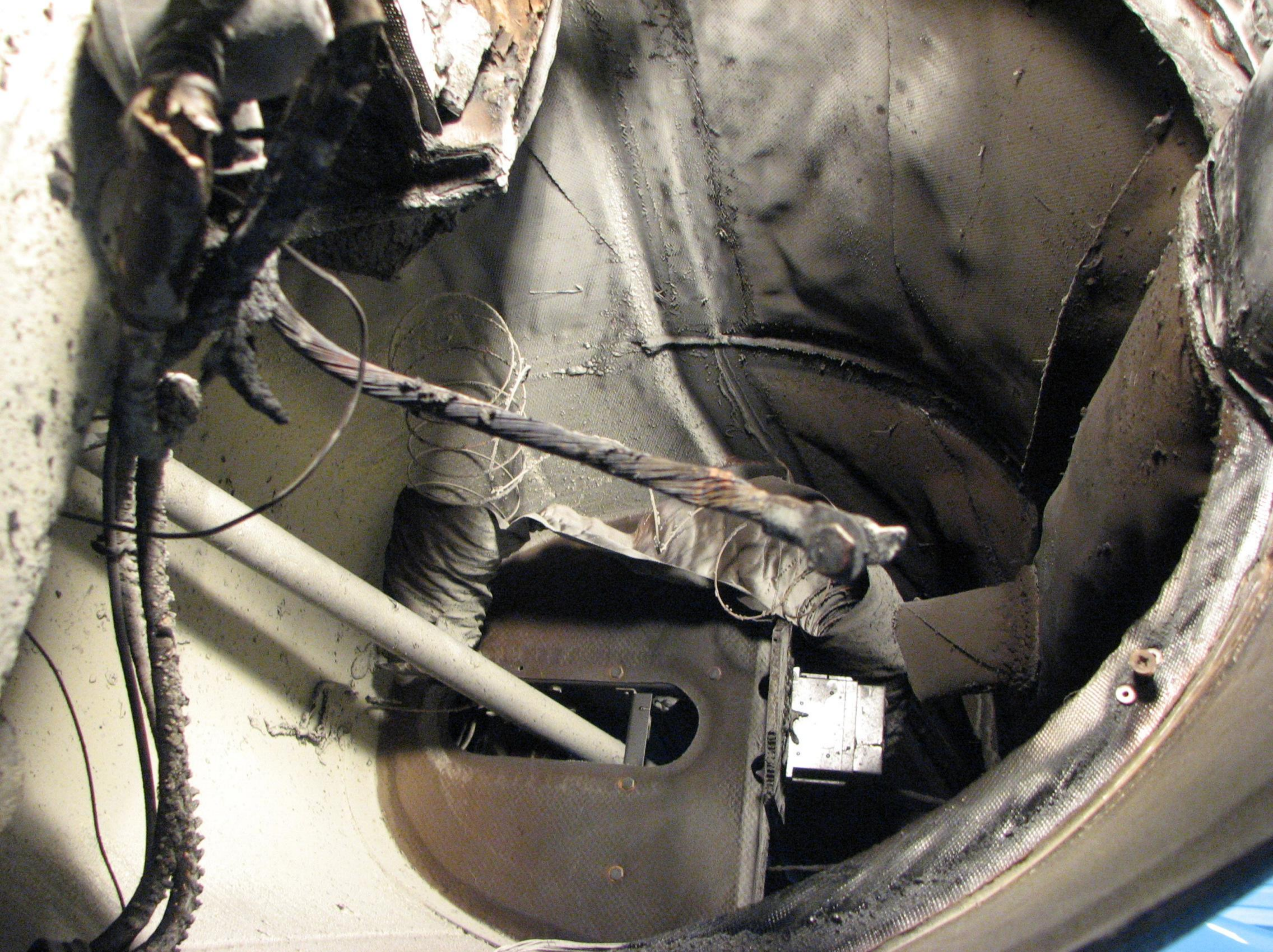
N731SJ Photograph of Internal Fuselage Damage
