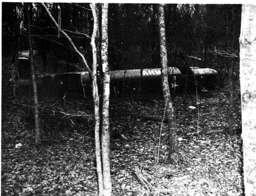
Figure 5. A side view of subject aircraft as it came to rest on its left side. The engine covers were removed after the accident.
