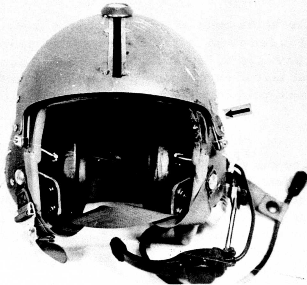
Figure 31. Front view of the copilot's helmet. The arrow denotes the impact area.
