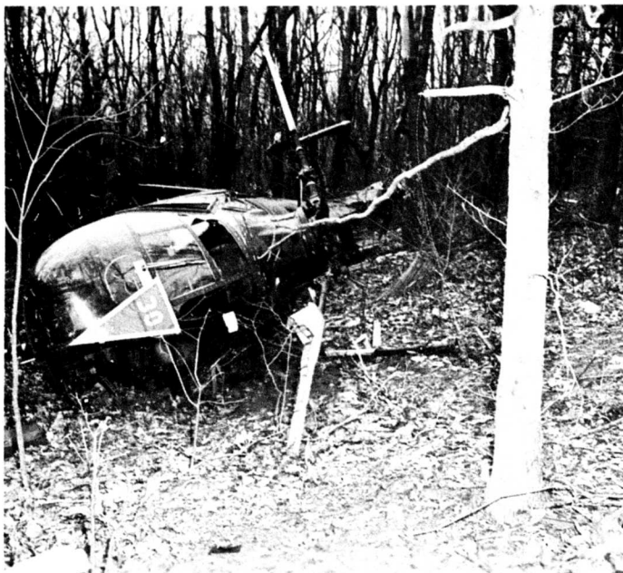
Figure 7. Front view of the helicopter showing the broken nose bubble on the left side.
