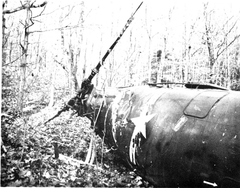
↑ Figure 9. A view of the aircraft looking toward the forward rotor. The arrows indicate the operable, but unused, ceiling emergency exits.
