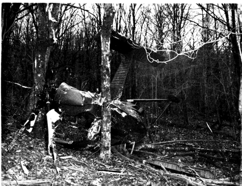
Figure 6. The nose-down attitude was caused by the aft end of the aircraft being wedged between several large trees as shown in the above photograph.
