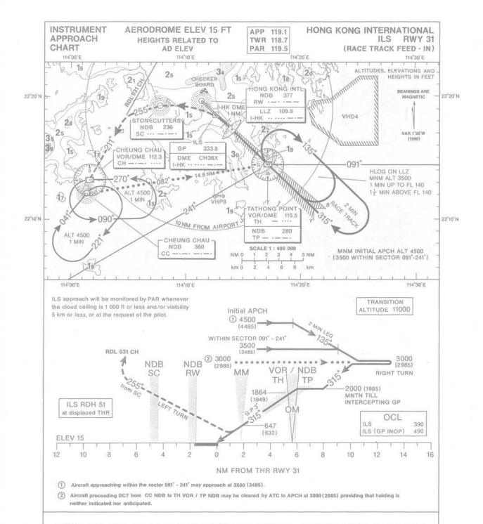
MISSED APPROACH: Climb to and maintain 2 500 ft on track 315°M towards 'RW' NDB. When passing within 1 NM southeast of 'I-HK' DME and above 330 ft, turn left to 'SC' NDB and continue climb to 4 500 ft. From 'SC' NDB track 255°M to intercept 'CH' VOR 031 radial. Turn left to track 211°M to 'CH' VOR and join the 'CH' VOR hold or as directed by ATC.
