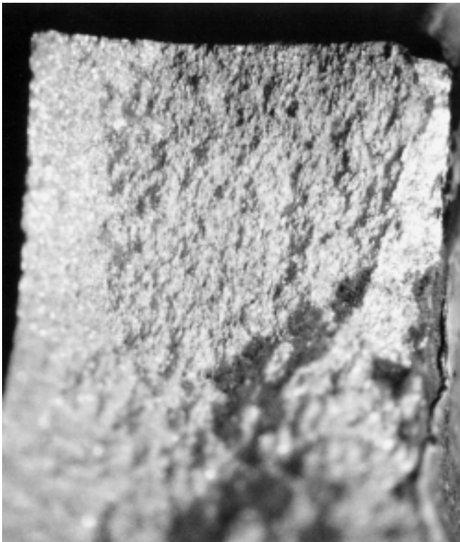
Figure 4B; magn. 16x Detail from figure 4A. The old "thumb-nail" shaped crack is surrounded by fresh overload cracking. The texture of the old crack reflects the forging material flow.
