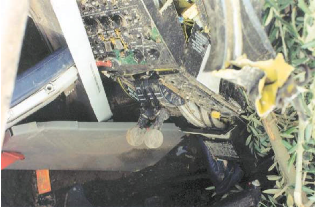
Photo 7.- Detail of the position of the power levers and engine switches on the ceiling panel. Right hand switch is in the "OFF" position.
