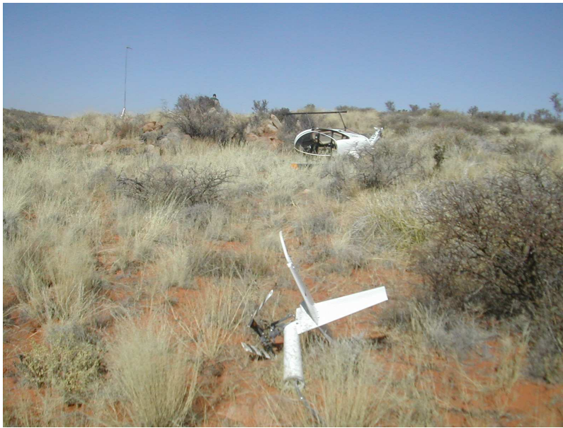
Figure 1: A view of the main wreckage and a section of the tail boom and rotor assembly
