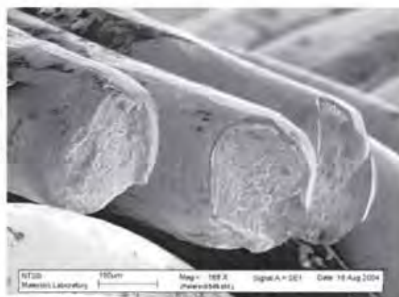
Fatigue fracture features observed on many wires
