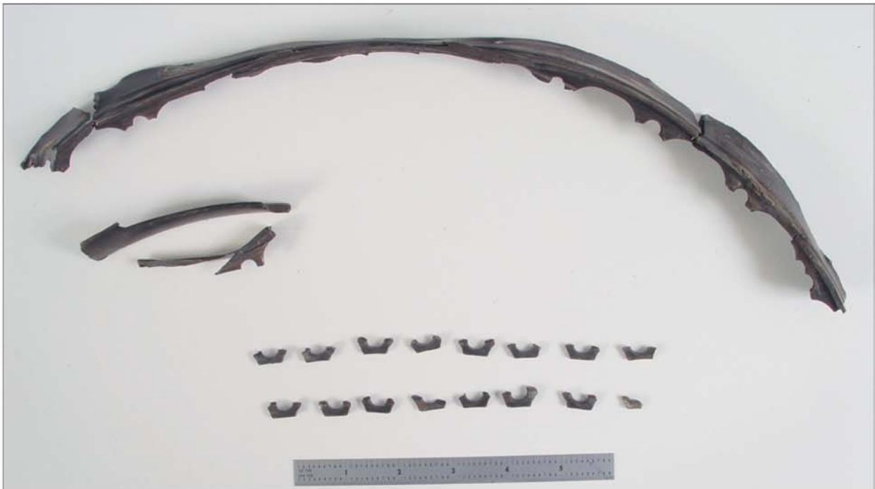
Figure 28. Fractured pieces of the skirt on the first stage HPT disk to which the rotating inner airseal was attached. View is of the forward side (looking aft).
