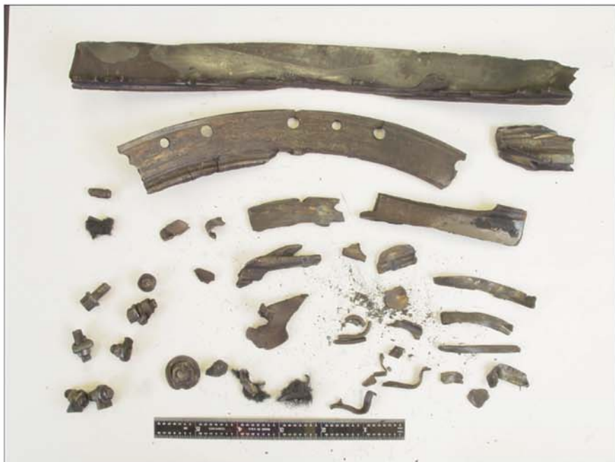
Figure 12. Overall view of the contents of the bag labeled "front face of 1st stage HPT hub".
