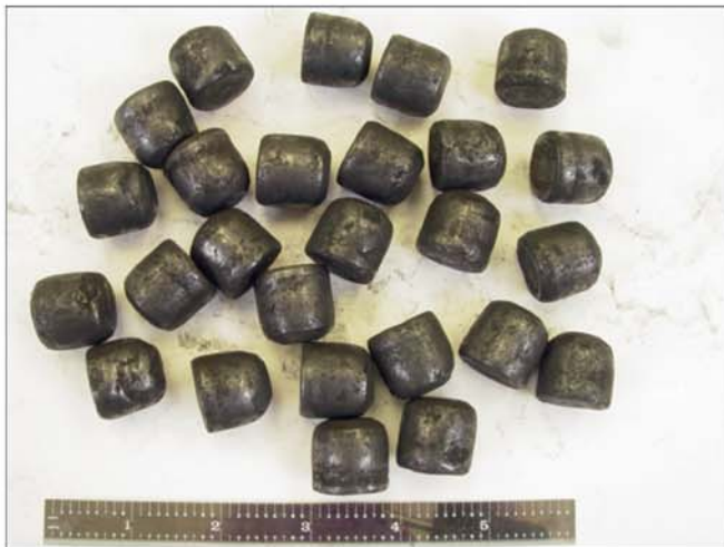
Figure 13. Overall view of the number 3 bearing rolling elements.
