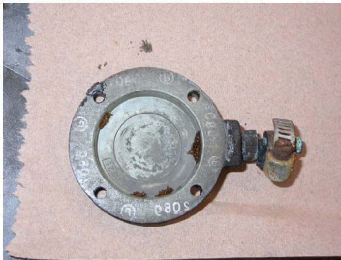
M/V cover with contamination. Ventilation tube inlet to the right.
