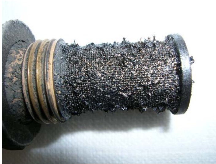
FCU filter with contamination
