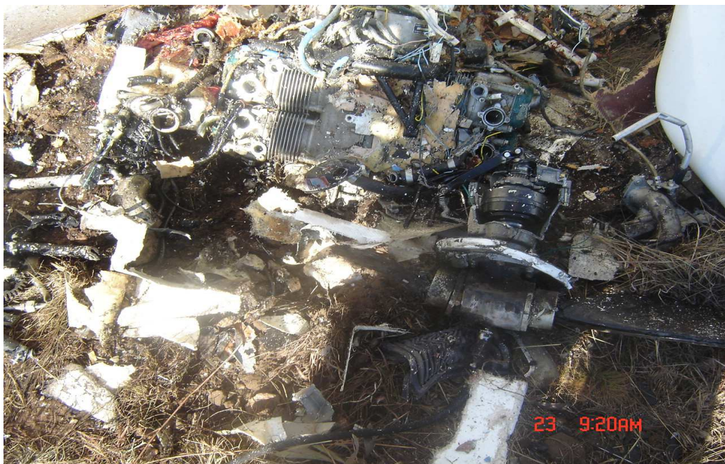
PHOTO 2: VIEW OF FRONT SECTION & ENGINE AFTER IMPACT WITH THE GROUND
