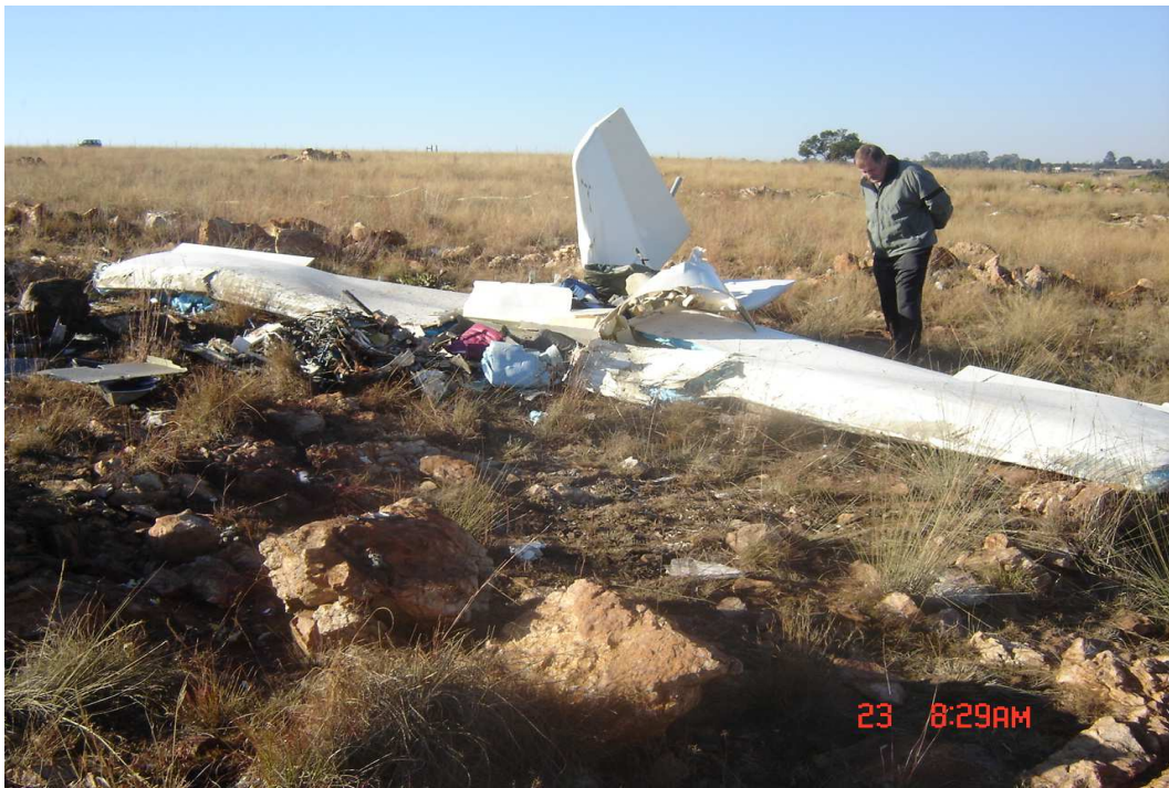
PHOTO 3: VIEW OF MAIN WRECKAGE AFTER IMPACT IN A NOSE-DOWN ATTITUDE IN ROCKY TERRAIN.
