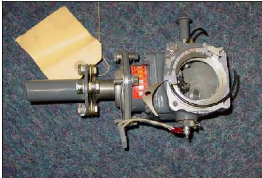
Figure 4: The fractured tail rotor gearbox in the as-supplied condition. Magnification: approximately 0,35x.
