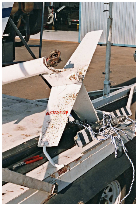
Figure 2: Damage to the tail rotor
