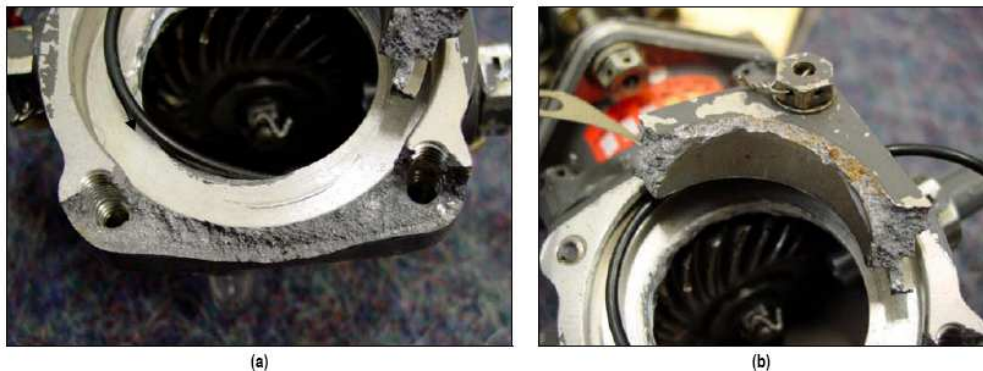
Figure 5: Enlarged views of the fracture surfaces on the tail rotor gearbox. Magnification: approximately 0,85x.
