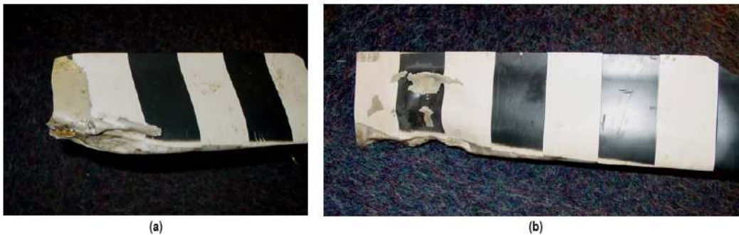
Figure 8: Damage observed on the tail rotor blades. Magnification: approximately 0,26x.
