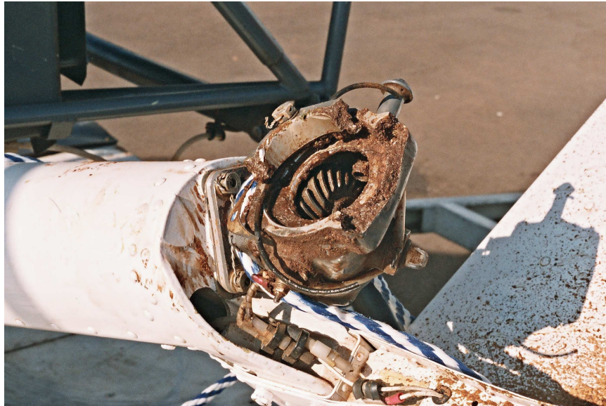
Figure 3: Damage to the tail rotor gearbox
