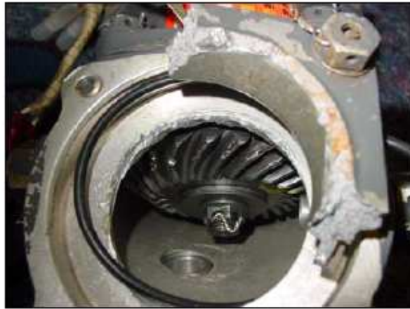
Figure 7: Chipped gear teeth. Magnification: 0,7x.
