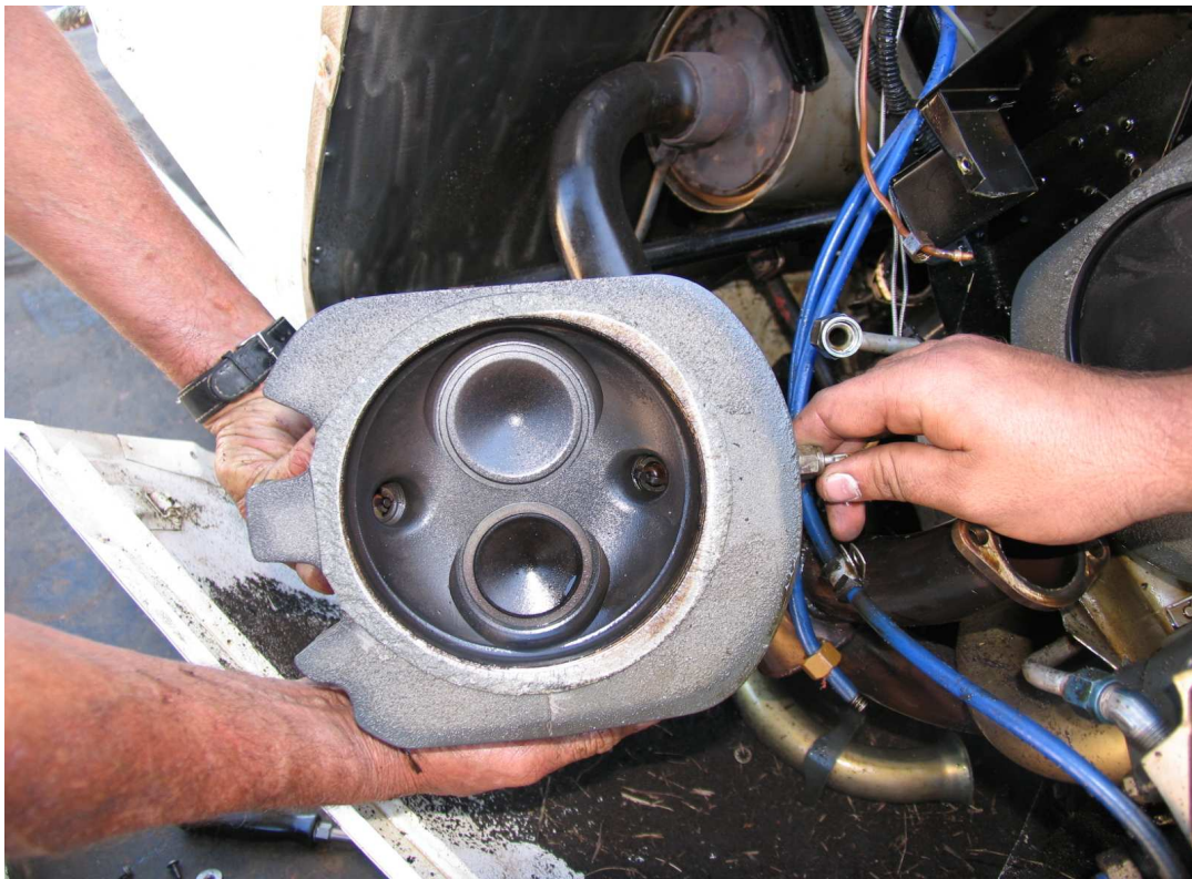
Figure 2: Fractured no. 2 cylinder head
