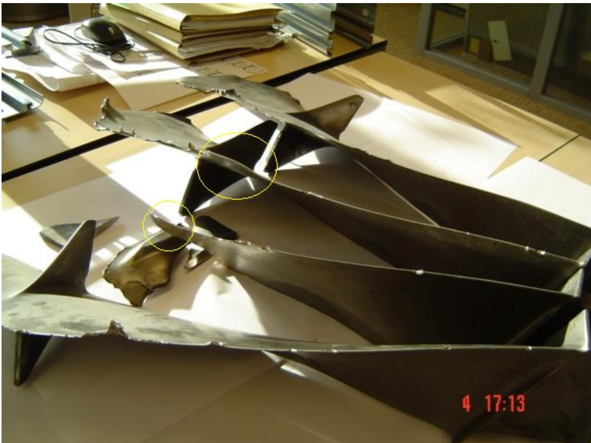
Figure 3: Cusps in leading edges of fan blades 1 and 38
