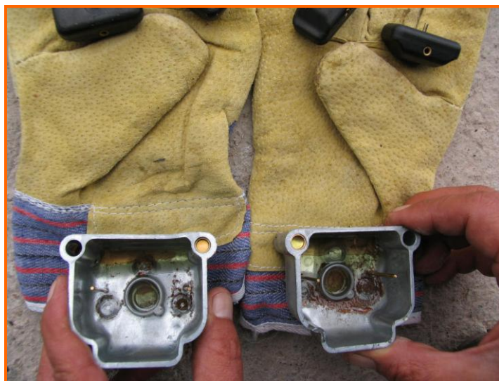
Figure 8: The carburettor fuel bowls, showing severe contamination
