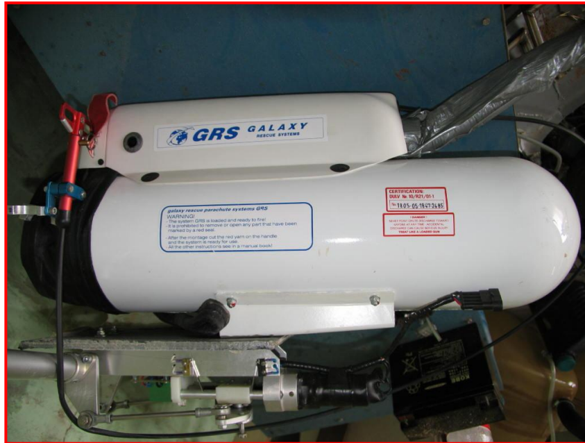
Figure 5: The ballistic parachute fitted to the aircraft
