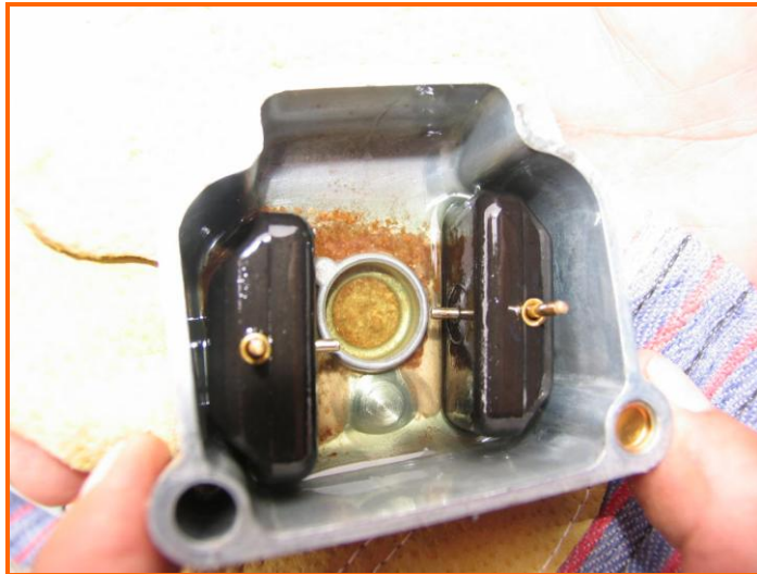
Figure 7: Contamination in the carburettor fuel bowl
