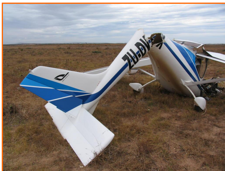
Figure 1: The main wreckage, showing the broken fuselage
