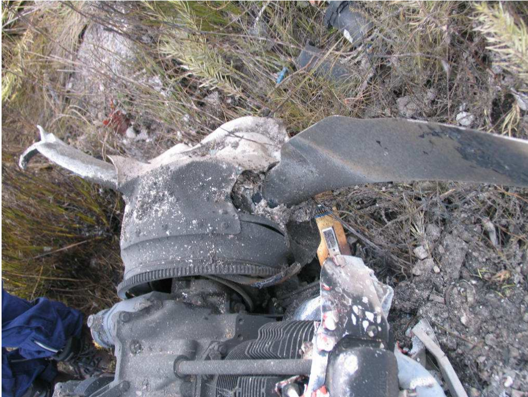
Figure 3: The propeller damage
