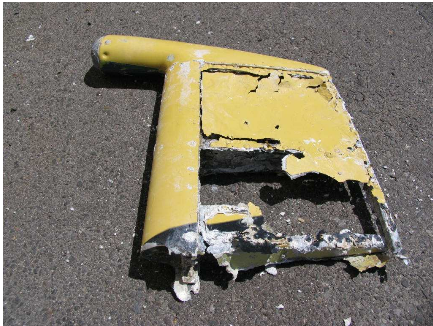
Figure 7: The outer section of the left elevator distorted by corrosion.
