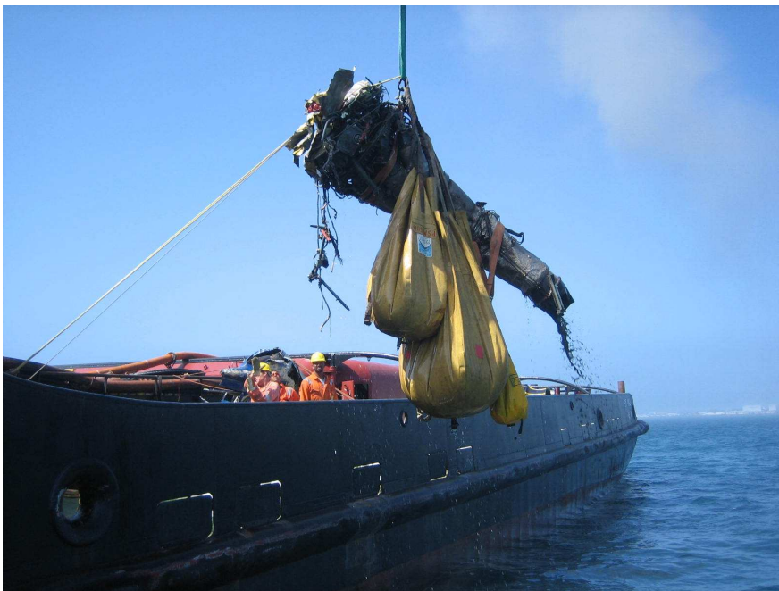
Figure 8: The engine being lifted by crane from the sea onto a special recovery vessel (ZTUG).
