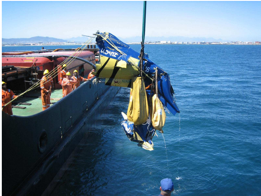
Figure 6: Recovery of the empennage section from the water onto the support vessel.
