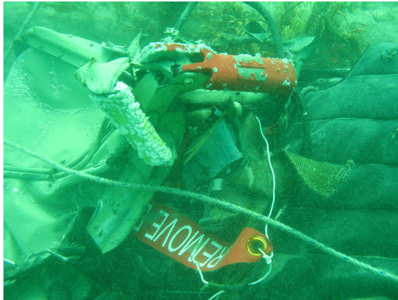
Figure 4: Underwater photo of the aft cockpit ejection seat with some of the pins still secure.
