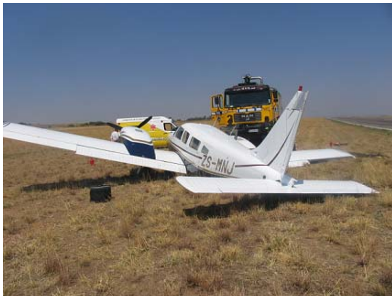
R/H main gear collapsed after landing
