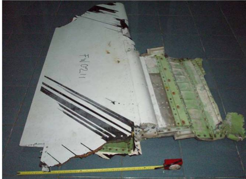
Figure A3: Part of Left Elevator showing upper surface. Found floating in the sea off the coast near Pare-Pare
