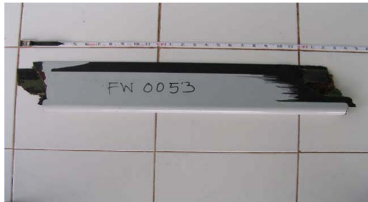
Figure A6 : Part of elevator tab. Found floating in the sea around Pare-pare
