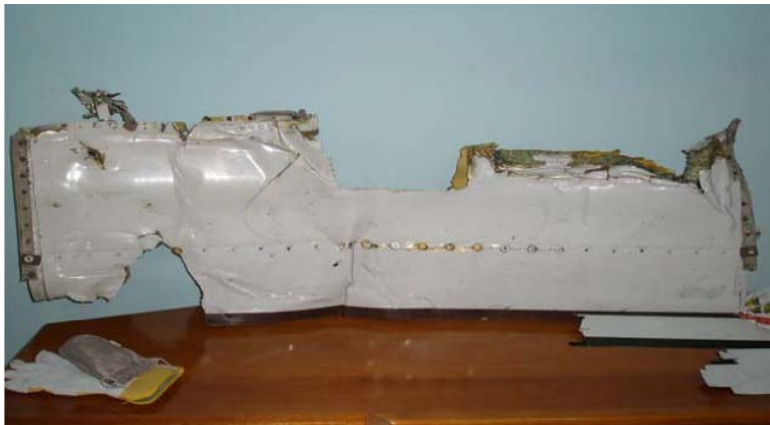
Figure A7 : Flight spoiler (showing lower surface) found floating in the sea off the coast of Pare-pare
