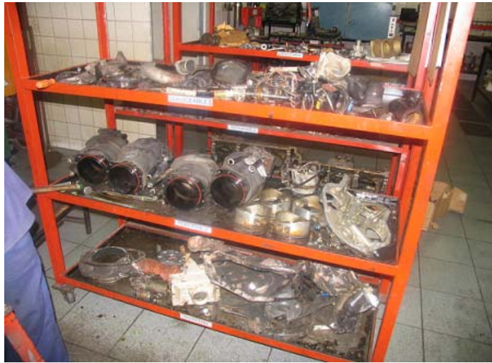
Disassembled Engine Parts stored on trolley after the “tear – down” inspection
