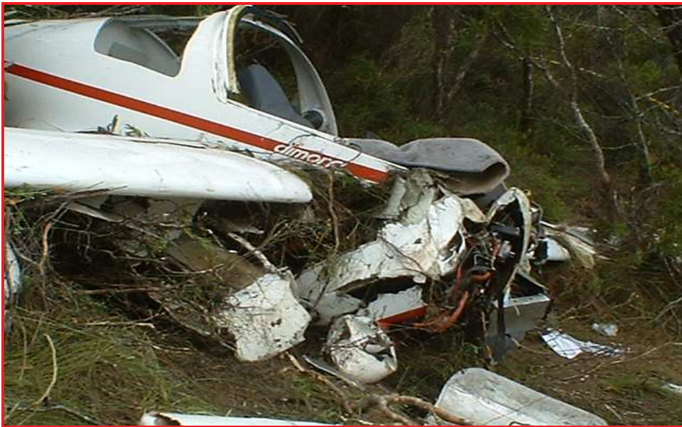
Figure 2. The extensive damage to the cockpit area.
