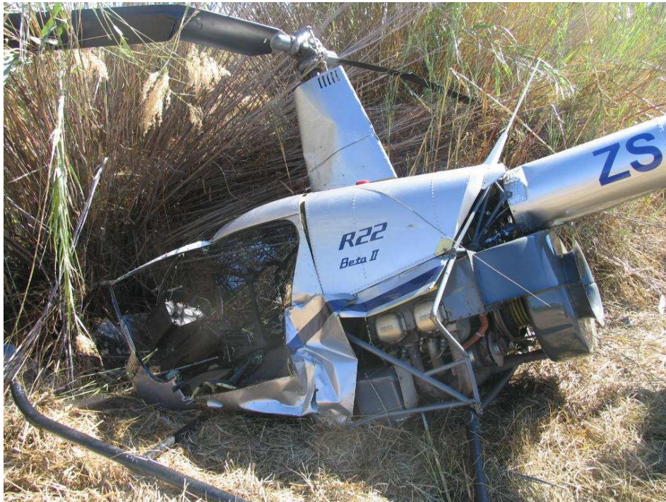
Figure 2. The extensive damage to the cabin.
