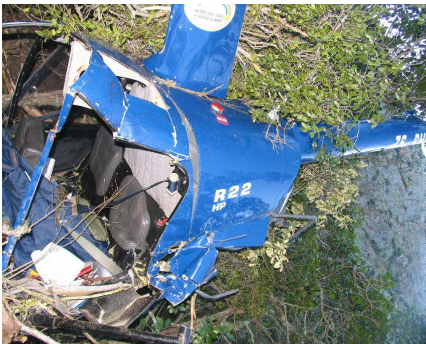
Figure 4: The helicopter wreckage, extensively damaged on impact with trees
