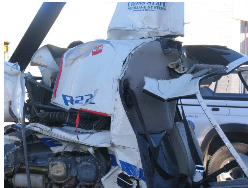
Photo 2 damage to the starboard side of the helicopter.
