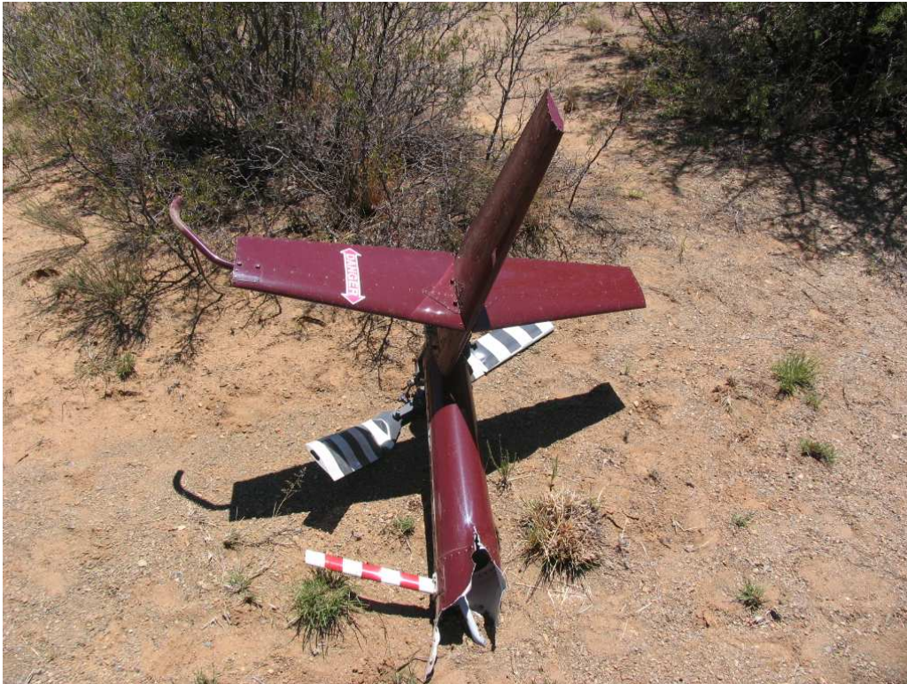
Figure 3. The severed tail boom.
