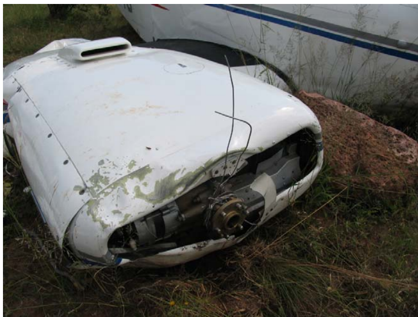
Figure 6. A view of the crankshaft flange with some electrical wire entangled around it.
