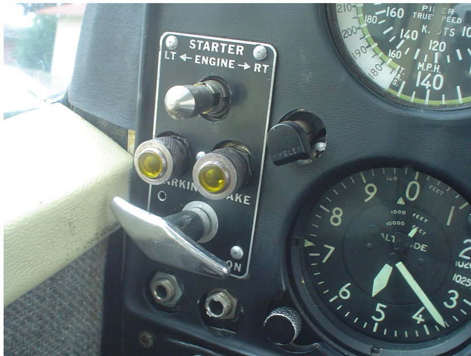
Figure 10: The park brake was found released and not applied
