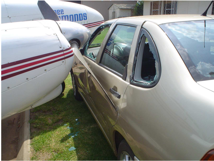
Figure 3: Damage to the right-hand propeller
