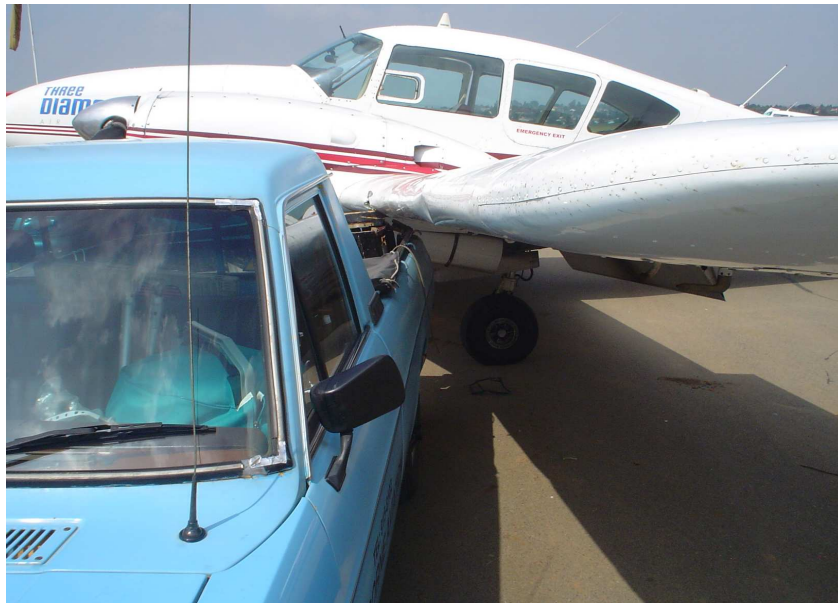
Figure 1: Damage to the left-hand wing leading edge
