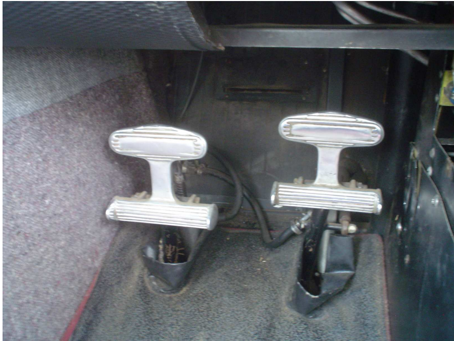
Figure 9: The on-site investigation revealed that the right rudder/brake pedal was in a slightly forward position
