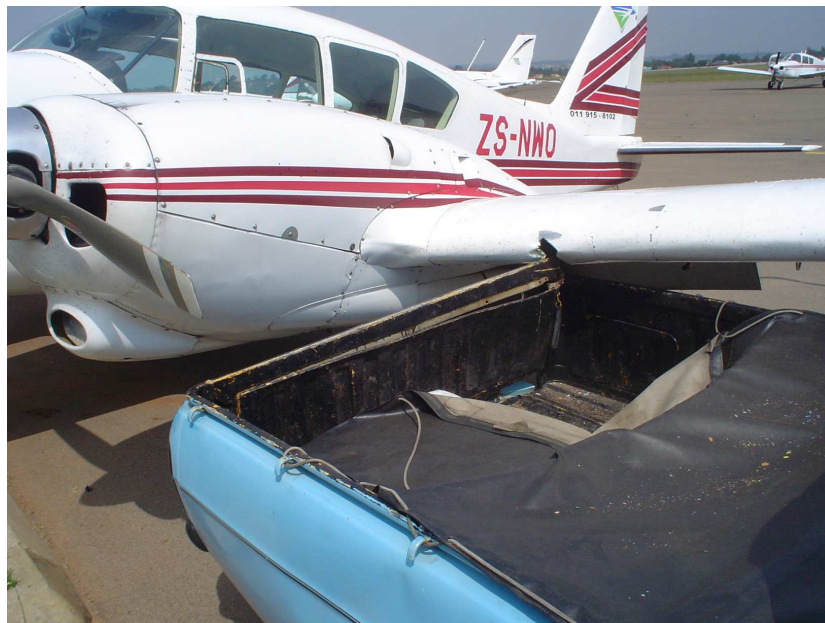
Figure 2: Damage to the left-hand wing's skin
