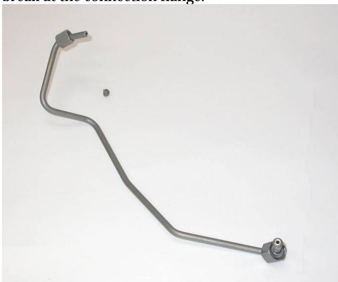
The fuel pipe is about 40 cm long and only secured by collar nuts at each end.
