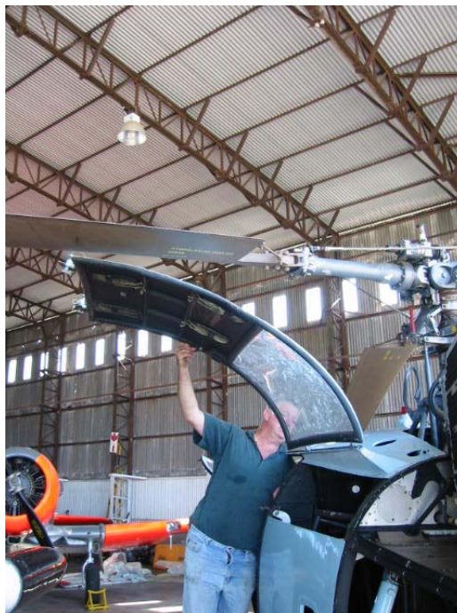
Photo 2. View of aft left sliding door deflected upwards towards the main rotor blades.
