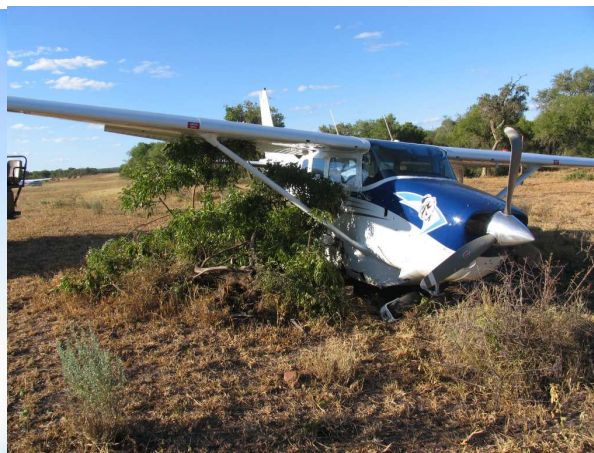
Figure 2: The aircraft in a nose-down attitude following nose landing gear separation
