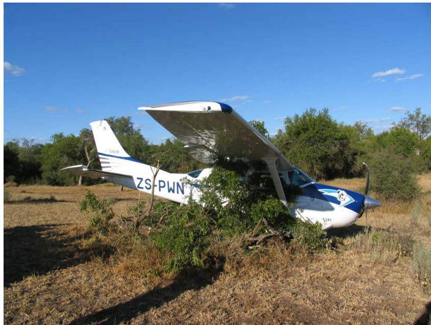
Figure 6: The aircraft it collided with a tree and the nose wheel collapsed
