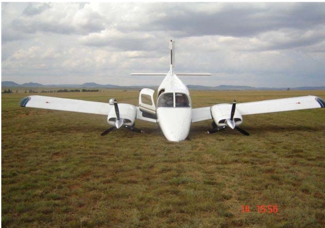
PHOTO 1: A/C NOSE LANDING GEAR COLLAPSED DURING TAXI ON GRASS.
