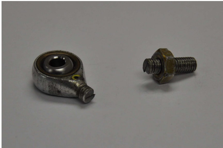
Figure 3. The failed throttle linkage – part no. A759-1.
