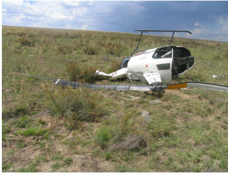
Figure 1: The main wreckage with the tail boom severed.
