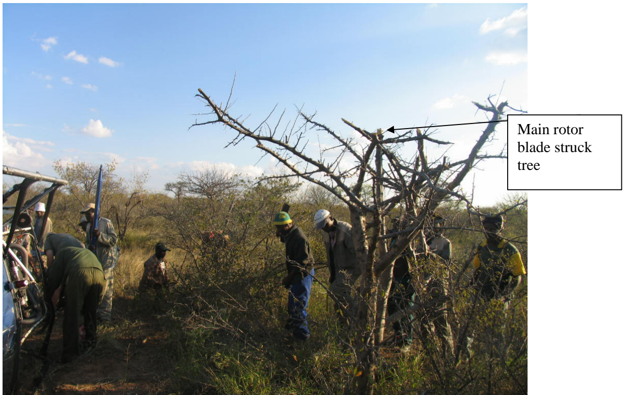
Fig 3: Main rotor struck a thorn tree
