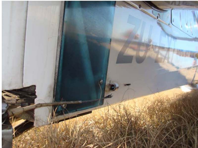
Figure 2. A view of the failed right rudder cable in the area of the fairlead.
