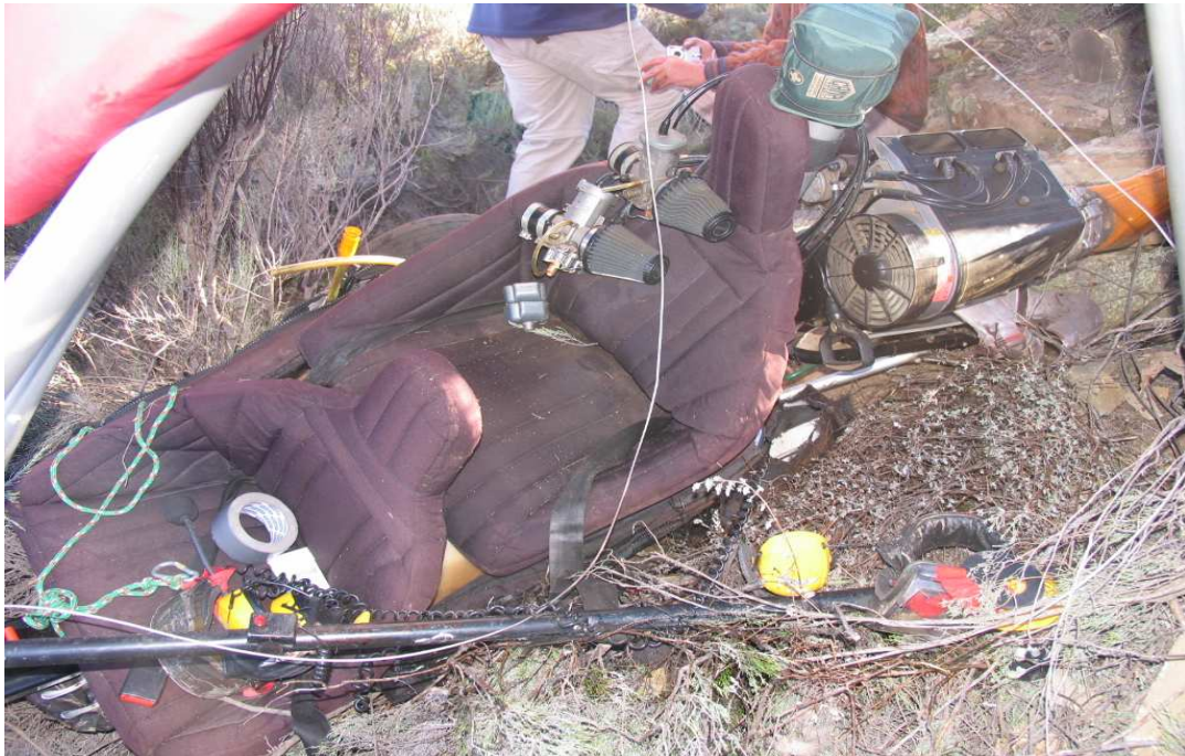
Photo 4: Seats and engine underneath canopy
