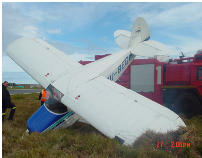
Photo: Left side wingtip digging into the ground.
