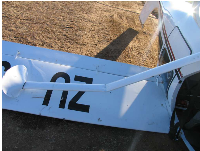
Figure 3. Visible damage to the left wing strut.
