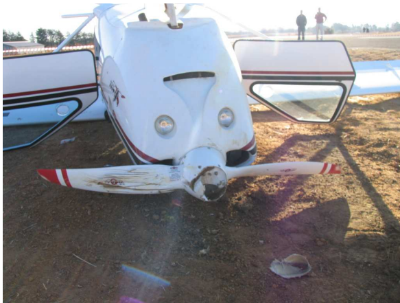
Figure 1. Indicating damage to the spinner and propeller.
