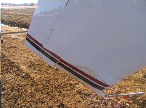
Figure 2. Damage to the vertical fin.
