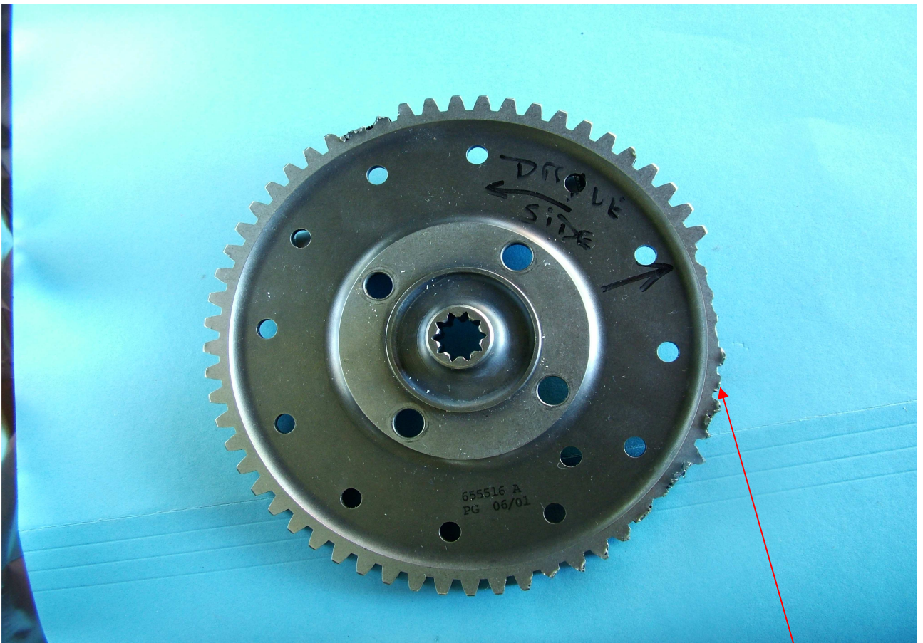
Picture 3: showing cam drive gear with failed teeth
