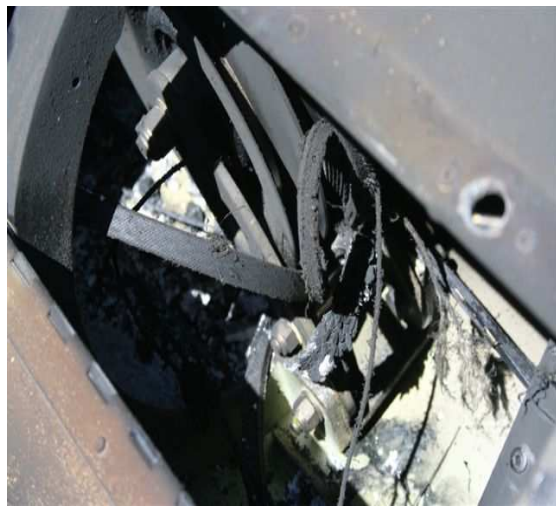
Figure 2. Views of the damaged tail rotor drive-belt.
