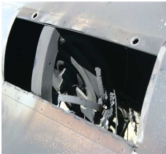
Figure 2. Views of the damaged tail rotor drive-belt.
