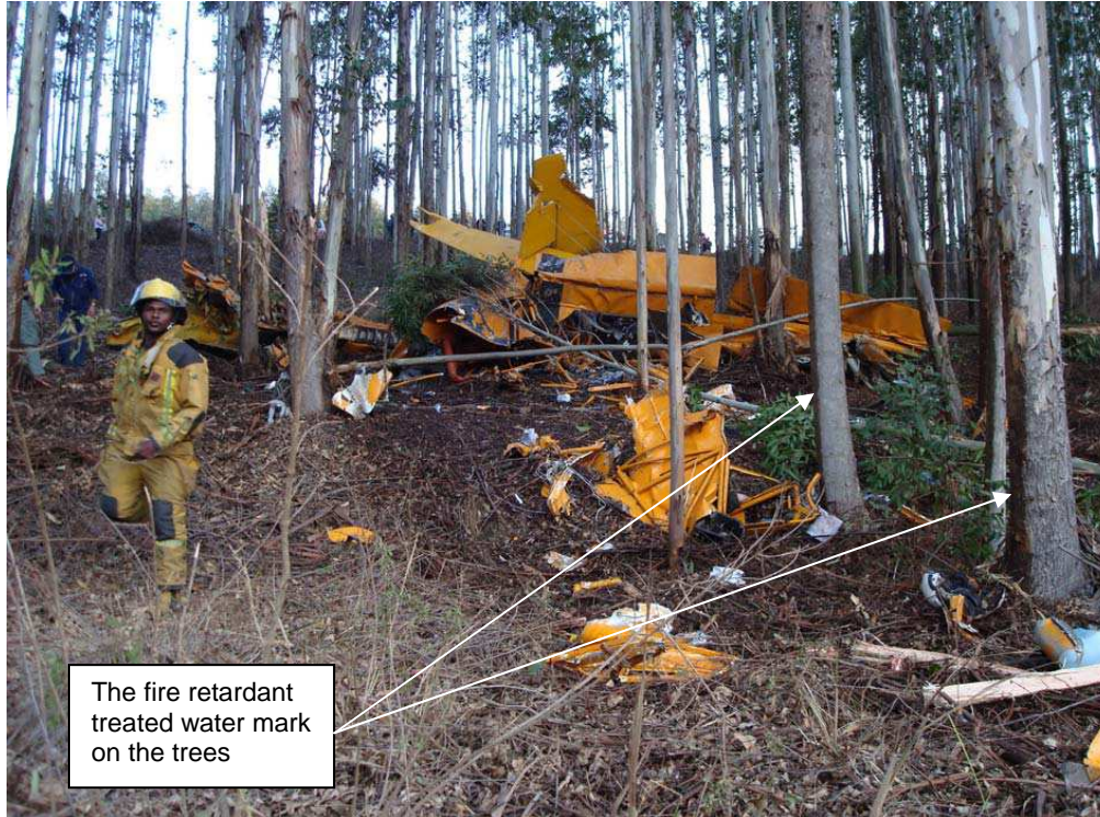
Photo 6: View of fire retardant treated water at the wreckage after the water load burst at impact The photo was taken minutes after the accident occurred
