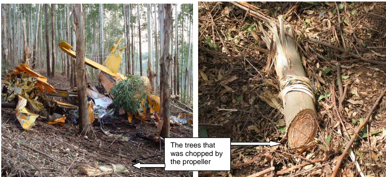
Photo 7 & Photo 8: View of the trees that was chopped by the propeller
