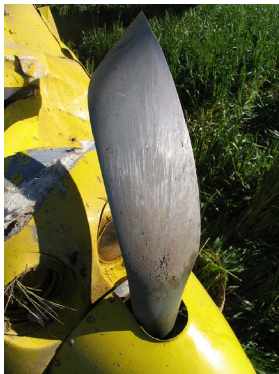
Figure 3 Scoring marks on the blades.
