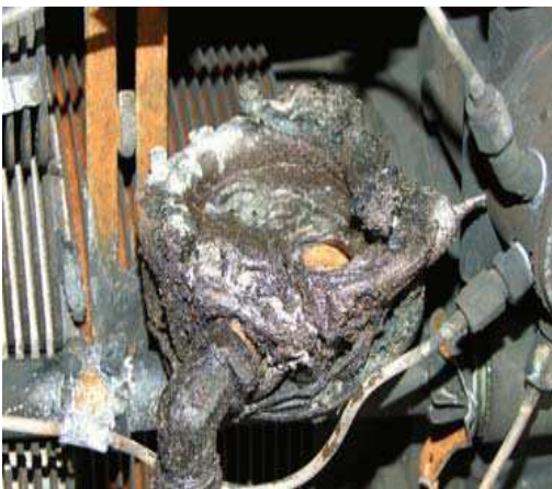
PHOTOS: The AC type fuel pump was excessively damaged due to fire, so no further test or inspections were carried out. ( see attached photo )
