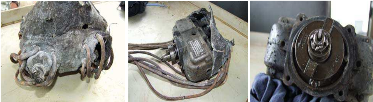
PHOTOS:The magneto was unable to be bench tested due to excessive fire damage, but no apparent defects due to failed parts was found.
