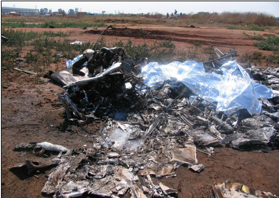
PHOTO2 : VIEW OF AIRCRAFT WRECKAGE DESTROYED BY THE POST-IMPACT FIRE
