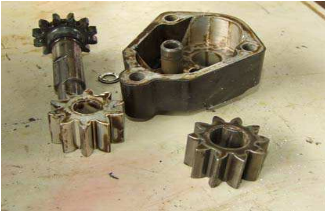
PHOTO: The oil pump was inspected and no internal damage found on gears , body and oil pump drive gear. ( see attached photo
