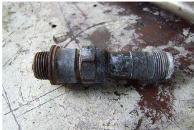
PHOTO :THE SPARK PLUGS RHM 40E WERE ALL FOUND INTACT AND IN PROPER WORKING ORDER
