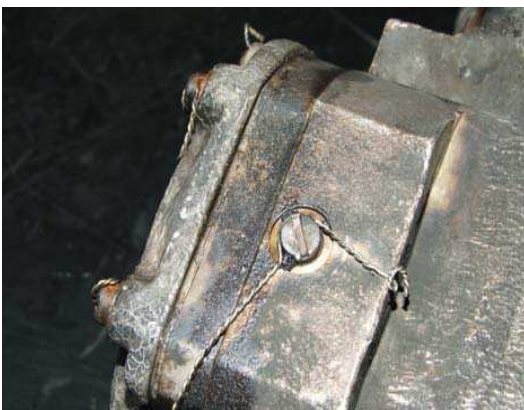
The Servo Unit s/n 59289 was not bench tested due to the heat damage that destroyed the fuel and air diaphragms
