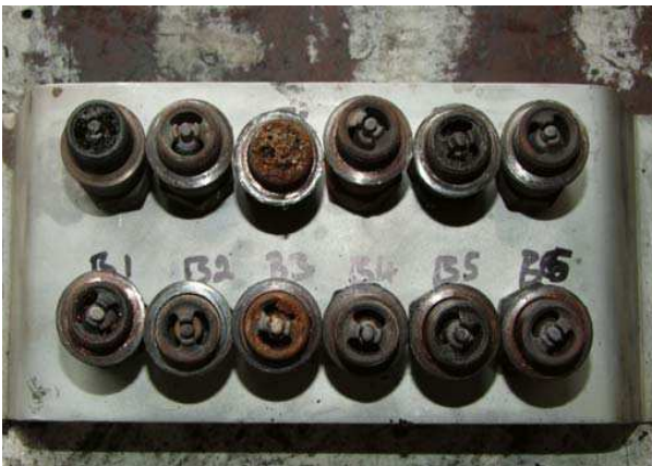
PHOTO :THE SPARK PLUGS RHM 40E WERE ALL FOUND INTACT AND IN PROPER WORKING ORDER
