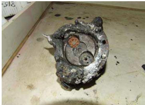
PHOTOS: The AC type fuel pump was excessively damaged due to fire, so no further test or inspections were carried out. ( see attached photo )
