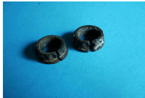
Photo showing cracked Crankcase thru bolt nuts.
