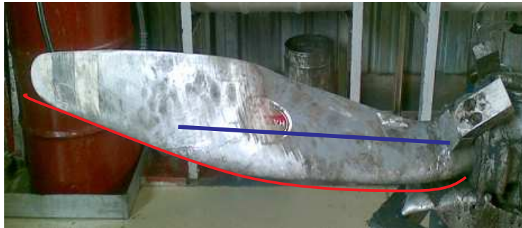
L/H propeller blade; Note scratches and slight curve in the plane of rotation, at the 6 inch station.
