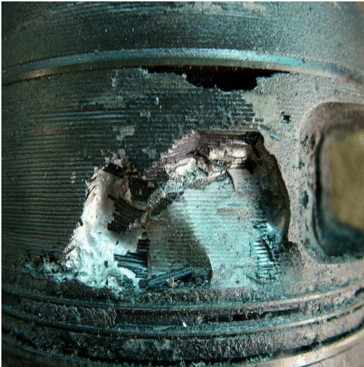
Photo showing damage caused to #5 piston.
