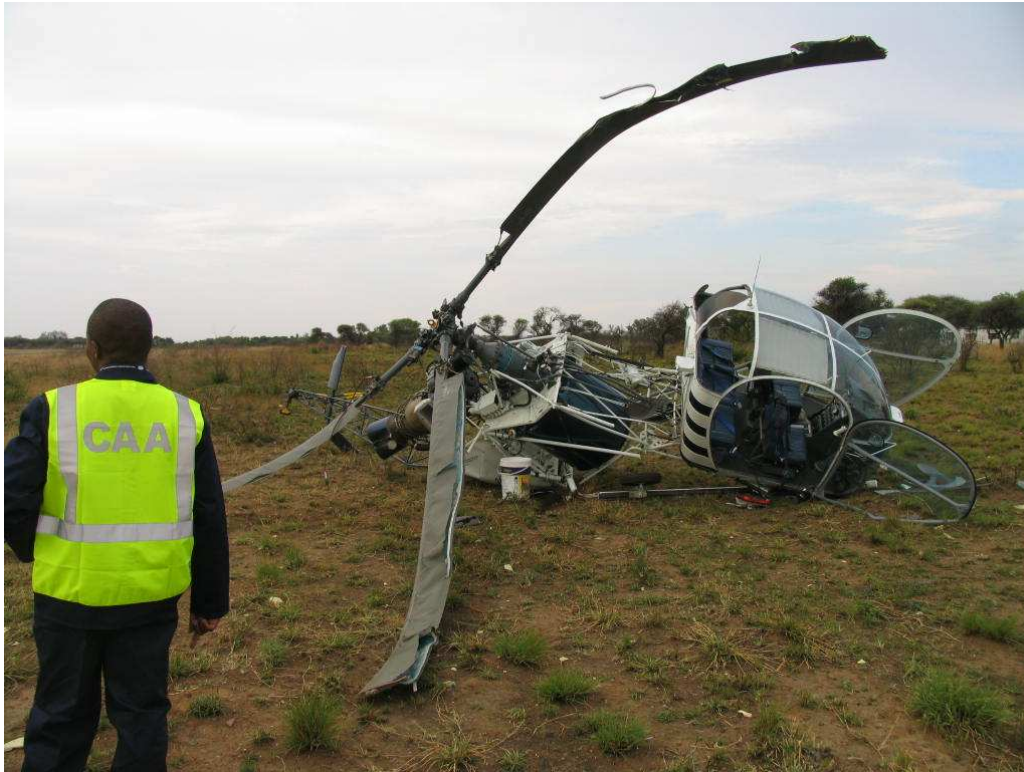
Figure 3: Damage sustained to main rotors and fuselage structure
