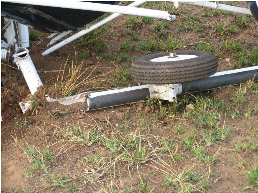
Figure 5: The helicopter skid damaged on impact
