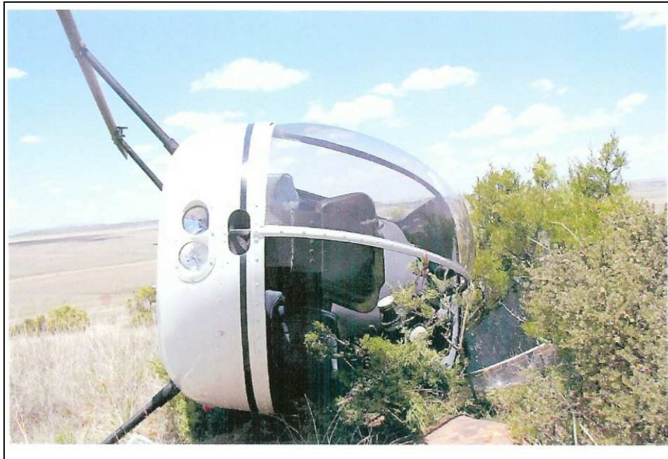
Figure 1. The helicopter after rolling over onto its left side.
