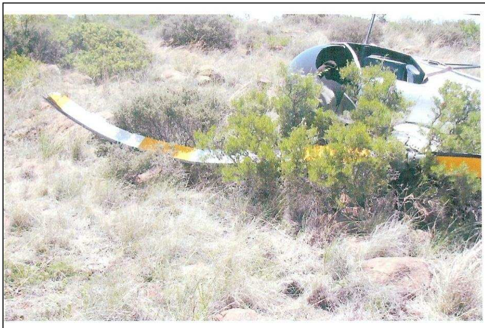
Figure 2. Damage to the main rotor.
