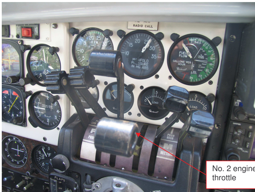
Figure 3: The number 2 engine throttle pulled backward/in the off position at the accident site
