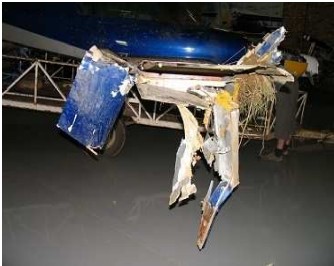
Figure 8 & 9, shows extent of damage caused to the wings.
