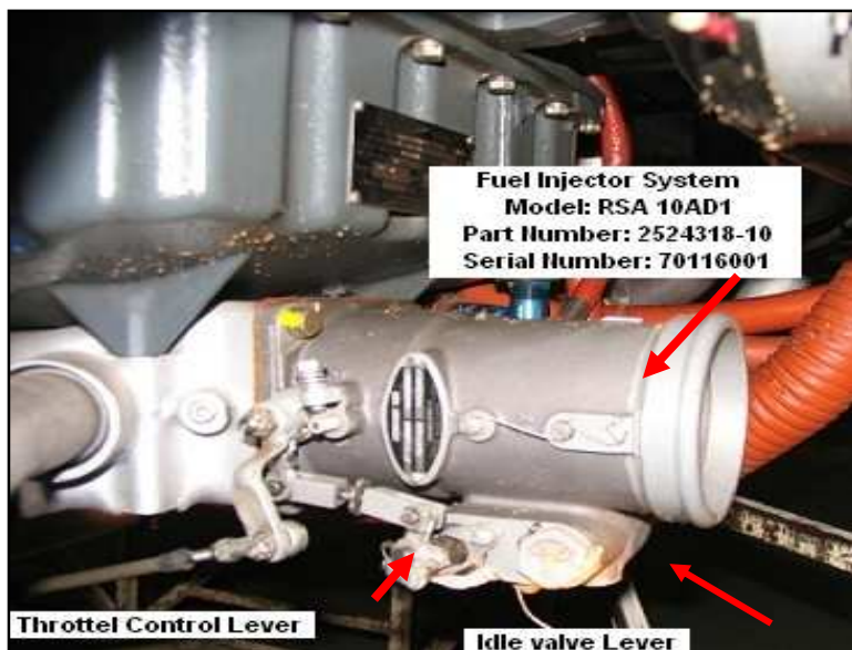
FIGURE 2: SHOWS THE FUEL INJECTOR INSTALLED TO THE ENGINE
