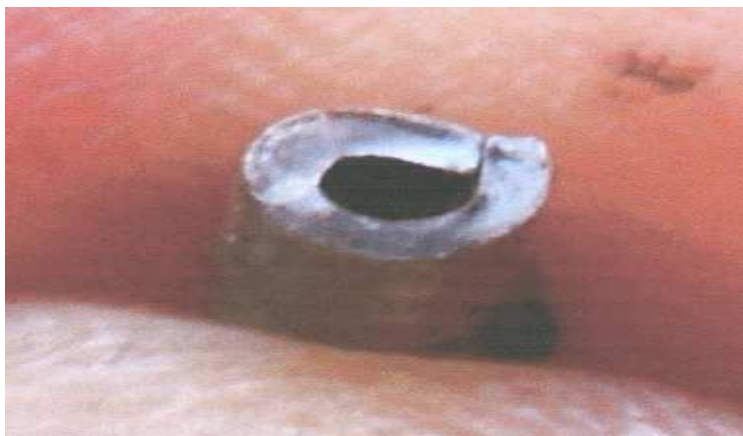
FIGURE 4: SHOWS THE SPRING STEEL ROLLED LOCKING PIN FAILURE
