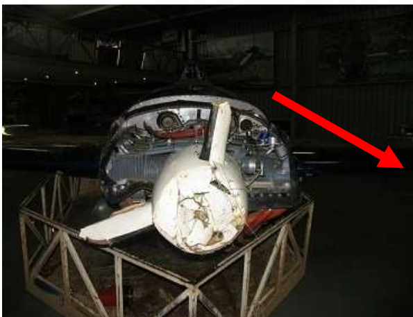
Figure 10, shows extend of damage caused to Propeller
