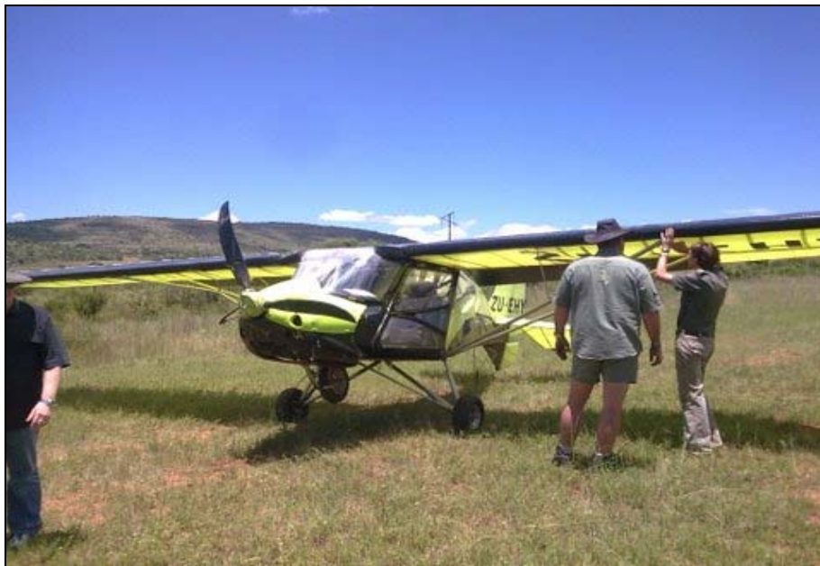
PHOTO 2: SHOWS AIRCRAFT POSITIONED BACK ONTO ITS MAIN WHEELS, PROPELLER BLADES BENT, RIGHT WING STRUT BENT & NOSE WHEEL DAMAGED.
