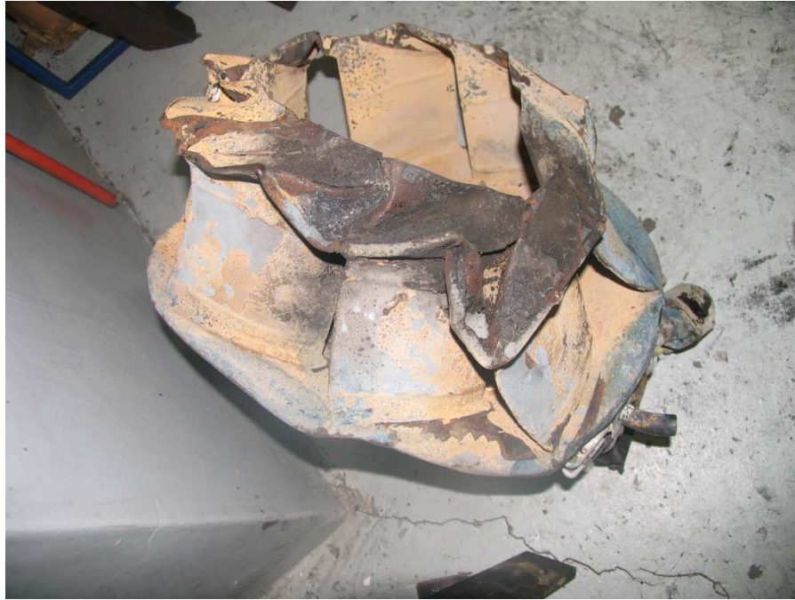
Figure 5: View of a deformed cooling fan.
