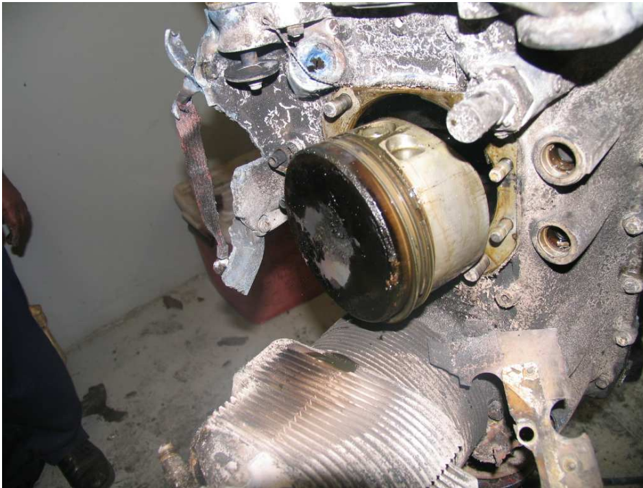
Figure 4: Heat damage caused to cylinders and pistons.
