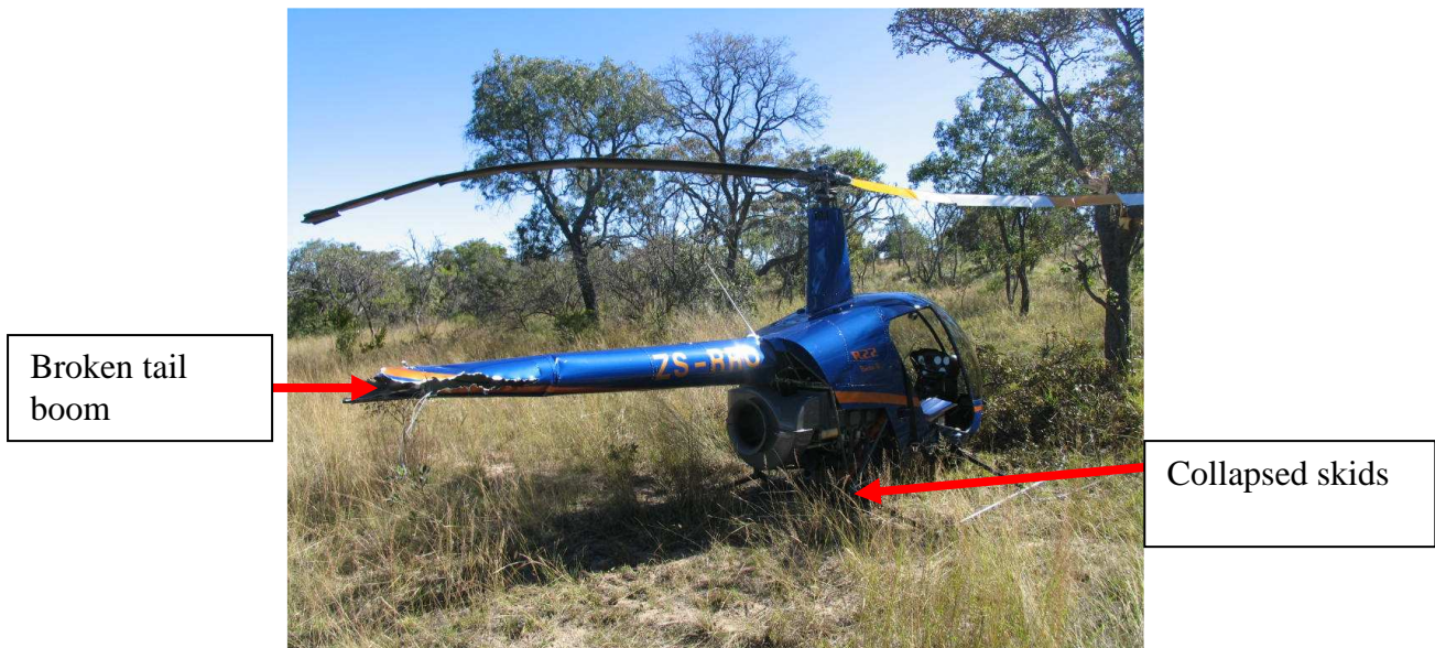
Figure 1: Damage to the tail boom and skids
